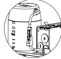
**Note:** Captive hooks are preinstalled for 1-3/8" (35 mm) ceiling thickness. Adjustment possibility up to a maximum of 2" (51 mm) ceiling thickness.
