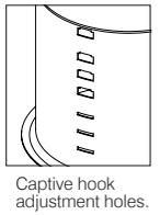
11. Lock the captive hooks and make sure the hooks apply a pressure against the ceiling to maintain the can firmly in place.
