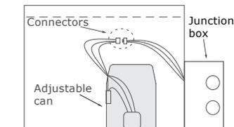
12. Insert the can into the mounting frame, pushing the fastening hooks through the lateral opening and secure the pot against the ceiling with the two adjustment screws.
