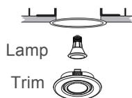
**Non orientable:** Screw the lamp in the housing. Fix the trim into the can.
