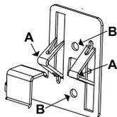
**Suspended ceiling:** Hang the mounting bars on the tee bars.
